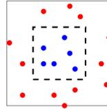
Assume that the probability distribution  $\mathcal{D}$  is such that instances are distributed uniformly within the gray square and the labeling function,  $f$ , determines the label to be 1 if the instance is within the inner blue square, and 0 otherwise. The area of the gray square in the picture is 2 and the area of the blue square is 1. Consider the following predictor:
