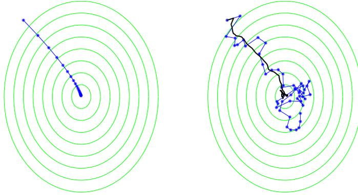
**Figure 14.3** An illustration of the gradient descent algorithm (left) and the stochastic gradient descent algorithm (right). The function to be minimized is  $1.25(x + 6)^2 + (y - 8)^2$ . For the stochastic case, the black line depicts the averaged value of  $\mathbf{w}$ .
