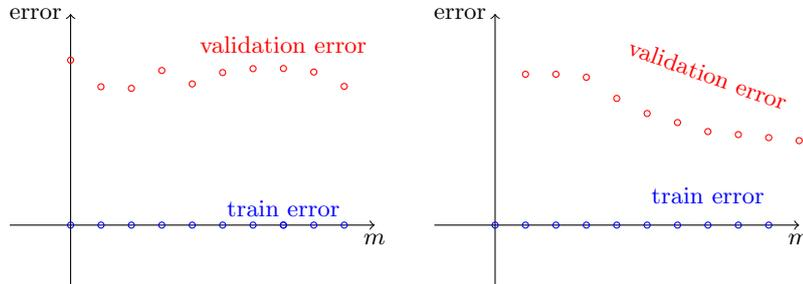
**Figure 11.1** Examples of learning curves. Left: This learning curve corresponds to the scenario in which the number of examples is always smaller than the VC dimension of the class. Right: This learning curve corresponds to the scenario in which the approximation error is zero and the number of examples is larger than the VC dimension of the class.
