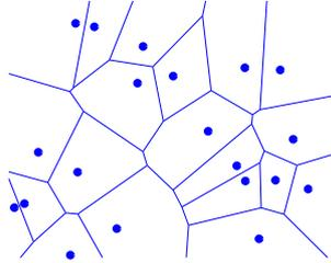
**Figure 19.1** An illustration of the decision boundaries of the 1-NN rule. The points depicted are the sample points, and the predicted label of any new point will be the label of the sample point in the center of the cell it belongs to. These cells are called a Voronoi Tessellation of the space.
